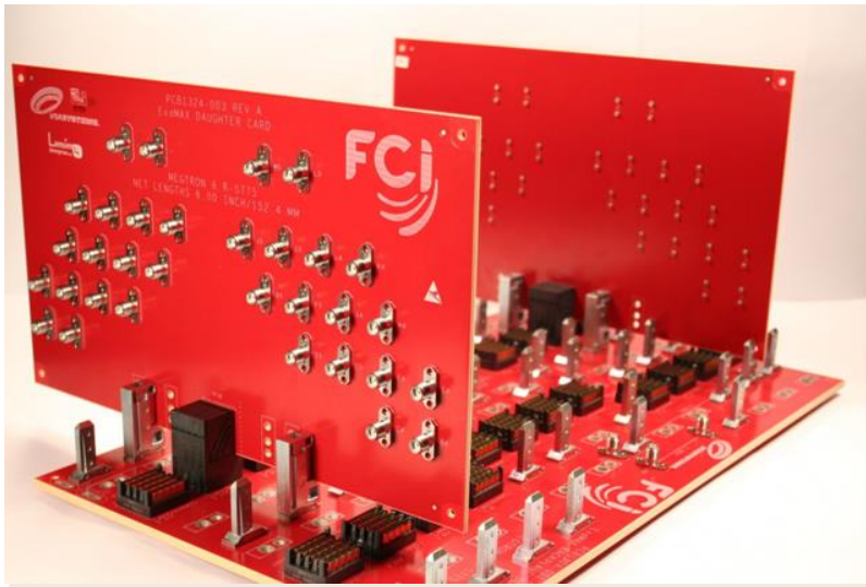
Figure 18 Amphenol-FCI Examax demo platform and channel topology summary used for case study.
